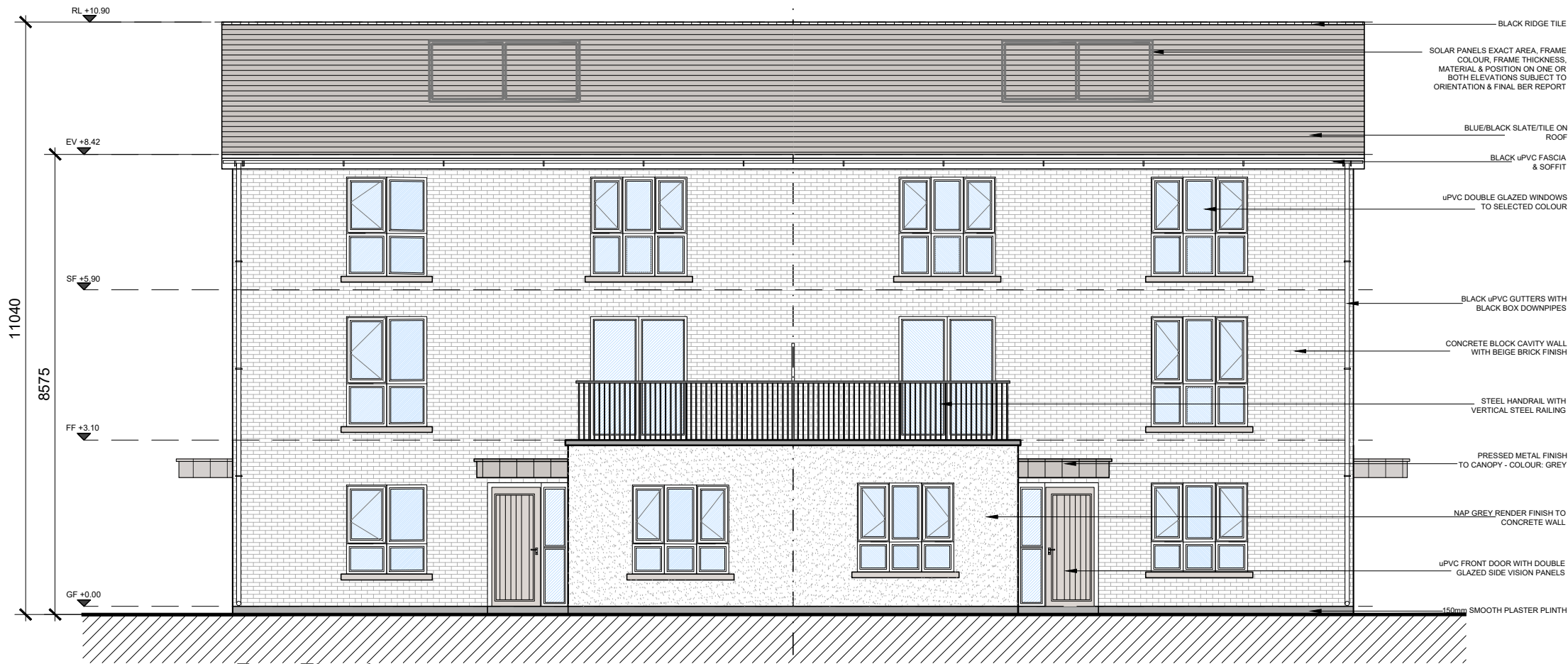
Front Elevation SCALE 1:100 @ A3
