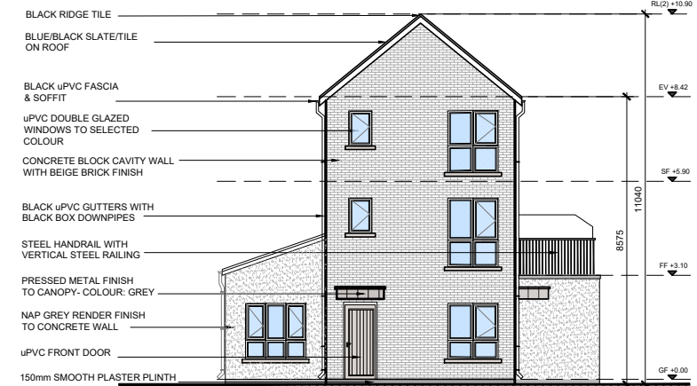
Side Elevations (G1/G3) SCALE 1:200 @ A3
